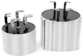
**kW power transformers** for PV inverters and traction applications are generally customised designs based on nanocrystalline ring cores which offer significantly higher saturation induction (1.2 Tesla) than ferrite cores in addition to low hysteresis loss. These properties deliver the advantages of lower weight and volume, enhanced efficiency and extended operating temperature range (up to 120 °C).
