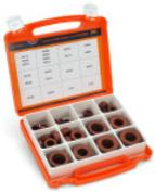
In the area of **nanocrystalline toroidal tape-wound cores**, the Core Sample Kit has been expanded to include VITROPERM<sup>®</sup> cores with external diameter up to 45 mm. The kit is suitable for the development of common mode chokes for rated current up to approx. 80 A and output of up to approx. 20 kW. The wide range of permeability levels  $\mu$  for each core size provides developers with the maximum flexibility in laboratory testing. The new kit is available from VAC distributors.
