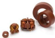
**kW power transformers** for PV inverters are based on nanocrystalline ring cores which offer significantly higher saturation induction (1.2 Tesla) than ferrite cores in addition to low hysteresis loss; these properties deliver the advantages of lower weight and volume, enhanced efficiency and extended operating temperature range (up to 120 °C). Power transformers are generally produced as custom designs.
